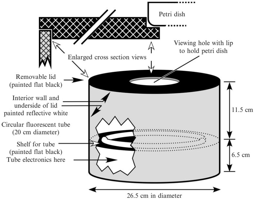
FIG. 2. Illuminator for viewing bacterial colonies in soft agar plates. The nature and dimensions of the stock material are provided in the text.
